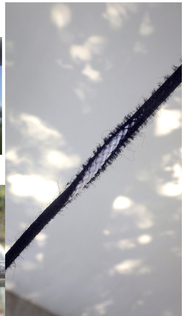
Support rope abraded by tree limb.
