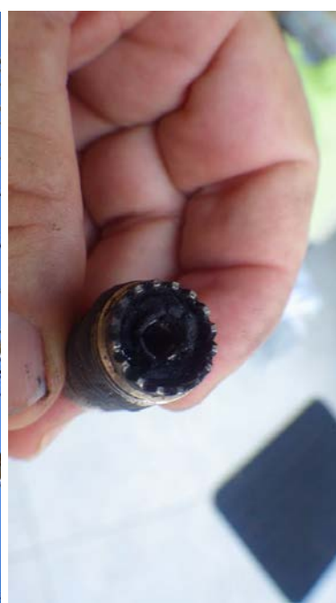
The blown-out PL-259 barrel which caused intermittent failure of the 2-element 80-meter wire beam pointed at the USA.
