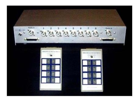
The RAS-8x2 provides flexible switching for your receiving antennas. Eight antennas can be routed to either of two radios, selected with remote keypads that fit easily into your shack. Preamp/filters for each radio provide 12 dB or more gain and filtering for 1.8-4.5 MHz (160M & 80M). When the preamps are OFF, the filters also are bypassed and the unit may be used on any frequency <0.5 MHz to 30 MHz.
