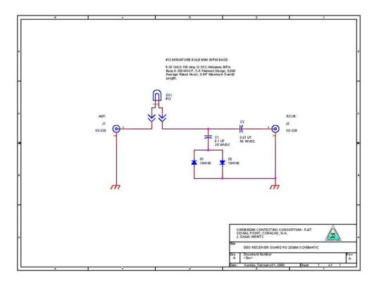
The RG-2000M uses a 6.3 V light bulb as the primary protective element. The idea is that as the tungsten filament heats from current flow, the resistance increases. Increasing resistance reduces the current flow, hopefully reaching a stable operating point where the resistance and current balance each other. This is the principle upon which all incandescent lamps operate. If that were not the case, light bulb filaments would simply vaporize when a voltage source is connected.
