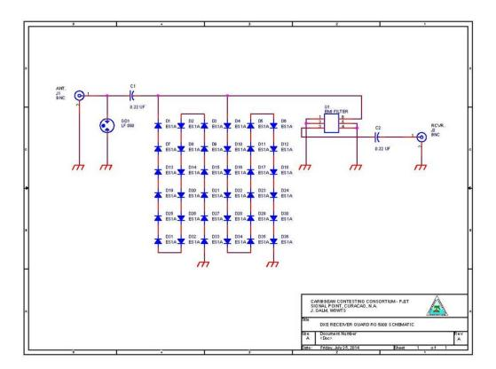
GD1 is a gas filled discharge tube. It is manufactured by Littlefuse, and is designed to change from insulating to conducting state when the terminal voltage rises about 90 V. Below 90 V, GD1 presents a very high resistance (several megohms) and a few picofarad of capacitance. The gas filling in discharge tubes at this voltage range is usually a mixture of Helium, Argon and Neon. When the electric field density across the gas mixture reaches a critical point, Townsend
