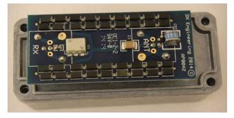
I was able to identify all of the parts in the RG-5000 except for the white, six pin gull wing surface mount device marked U1. The top of the package was filed off, removing all traces of the part markings. The RG-5000 circuit is as follows.
