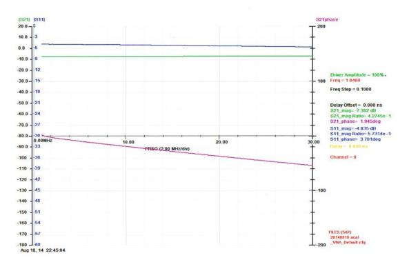
A similar forward gain and return loss sweep of the DX Engineering RG-5000 shows a very different picture.
