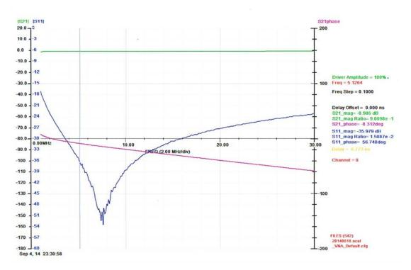
Forward gain S21 is nearly constant and close to 0 dB. This is as expected, since there is no filter or impedance in series with the signal path from antenna to receiver. In terms of impedance matching, the Antenna port is quite poor. S11 varies with frequency from -20 dB to less than -50 dB at some frequencies.
